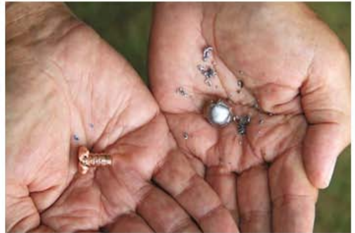
A copper bullet on the left and a lead bullet on the right after a shooting demonstration (Photo: Paul A. Smith / Milwaukee Journal Sentinel)
