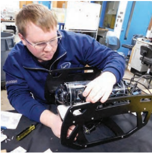
Above left, Hailey Greenleaf, a sophomore from Iron Mountain, Mich., tests the electronics enclosure for the WAM-V. At right, Nathan Van Antwerp, a junior from Reed City, Mich., working on the Remotely Operated Vehicle, (ROV) which is essentially an unmanned mini-submarine that can collect data underwater.
